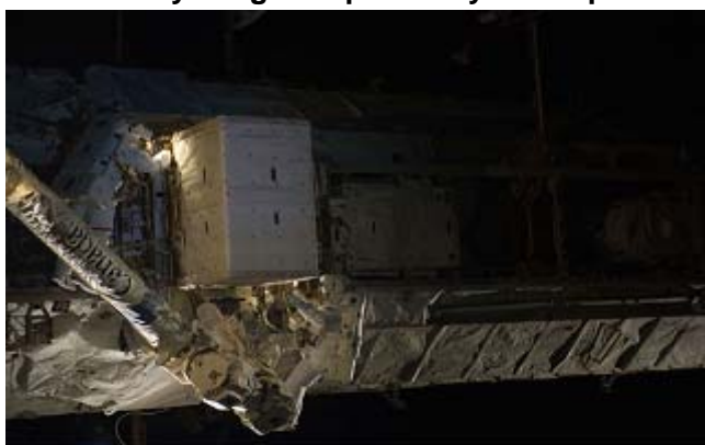
Image of extravehicular activities on the STS-131 mission. View of astronauts, as they work to tie down an Ammonia Tank Assembly on the International Space Station during STS-131 spacewalk.
